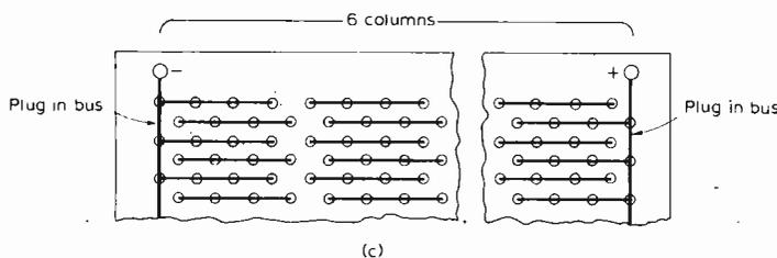
Fig. 1. Breadboard socket systems.
